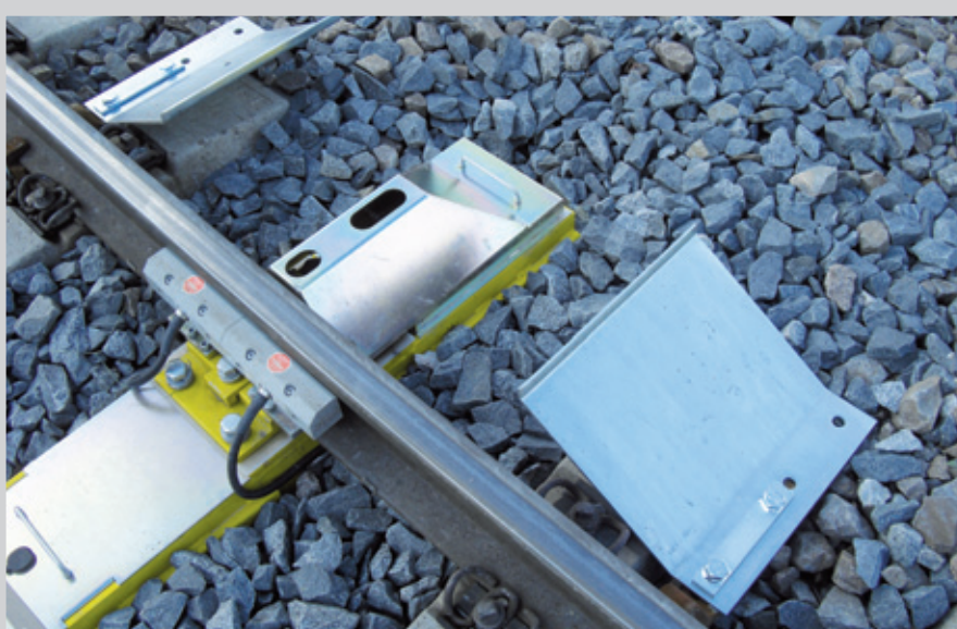
Figure 8: Hot axle box detector system controlled by wheel sensors
