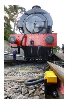
The Frauscher Wheel Sensor RSR123 proved to reliable detect even the old steam train's wheel flanges highly reliably.
