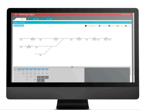
The Frauscher Diagnostic System FDS provides DFR's experts with remote access to real-time diagnostic data
